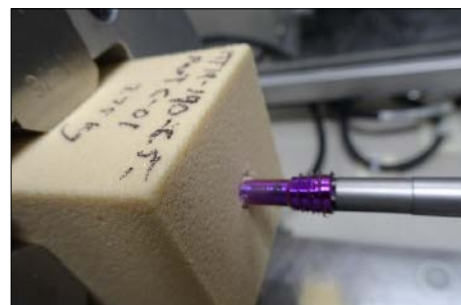
Figure 3: Representative test setup per ASTM F543 A4 (top); representative test setup per ASTM F543 A2 (middle); Representative post-test specimen (bottom)
