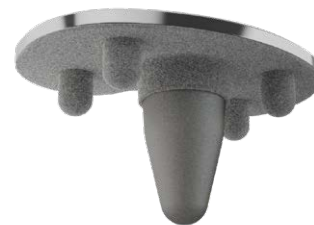
Figure 1: The ATTUNE ® Cementless RP Tibial Baseplate is designed with 4 pegs positioned radially from the central cone of the RP tibial base. The pegs and the underside of the ATTUNE Cementless RP Tibial Baseplate are coated in POROCOAT Porous Coating, with a grit blasted central keel
