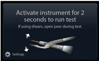
Connect the assembled Hand Piece and instrument to the generator and turn the generator power on. Follow On-Screen Instructions to complete initiation. The test prompt screen appears when the initiation sequence is complete. Activate the instrument (by depressing either one of the triggers) with the jaws open for 2 seconds to run test until the HARMONIC ® ready screen is displayed.
