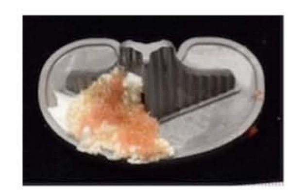
The above image demonstrated a mixed pattern of failure. There are areas where the implant-cement interface has failed adjacent to areas where the bone has failed. Lipid contamination of the tibial tray is also present.
