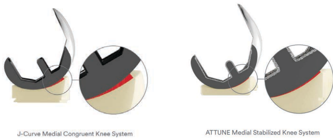
Figure 6. Images showing the anterior medial gap at 15 degrees of flexion in an ATTUNE™ Medial Stabilized Insert articulating with a ATTUNE GRADIUS™ Curve femoral geometry (right) and the Persona® Medial Congruent™ Bearing System insert articulating with the Multi-Radius Persona femur (left).
