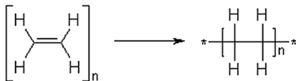
Fig. 1.1 Synthesis of polyethylene starting from ethylene monomer
